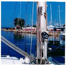
Loosen the halyard, pull reefing line through the stopper, tide the reefing line on the boom as fast as you can, hoist the main halyard. The main sheet goes from the boom end to the foot of the missan.
