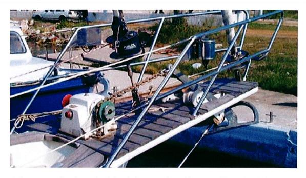
Only one way electric - to haul the chain, press the red button and keep the chain free from blocking in the locker.
